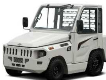
IC(Diesel) X Series Kapasitas 2.0~3.0t
