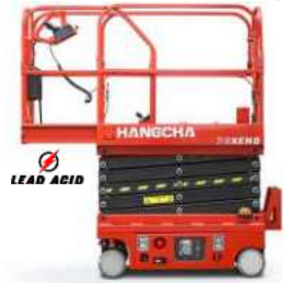
XB Series Pallet Truck With Scissor Lifts Kapasitas 500~2000Kg
